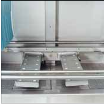
The water is sprayed from above and below, effectively covering the whole basket. The large washing compartment is easy to clean.
