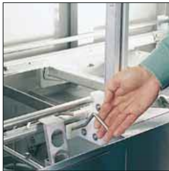
All the tanks can be emptied by pressing a lever. The bottom seals and level pipes are closed automatically when the machine is about to fill.
