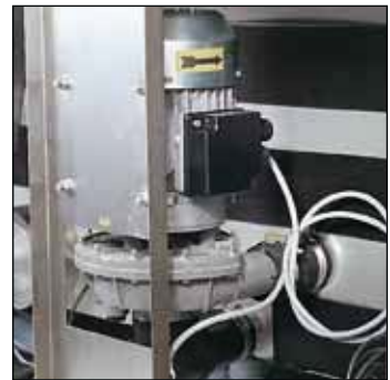
Self-emptying pumps in the washing and rinsing zones improve hygiene levels.
